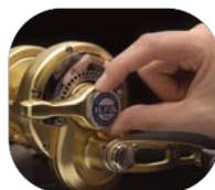
Step 3 Seat and thread on the new cam
